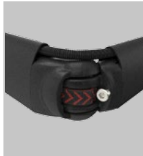
bionic tendon and cable conduit hidden in the arms
